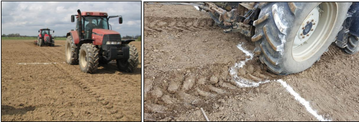
Fig. 2. Tire contact area influenced slip and soil disturbance, tractor loaded with draft
